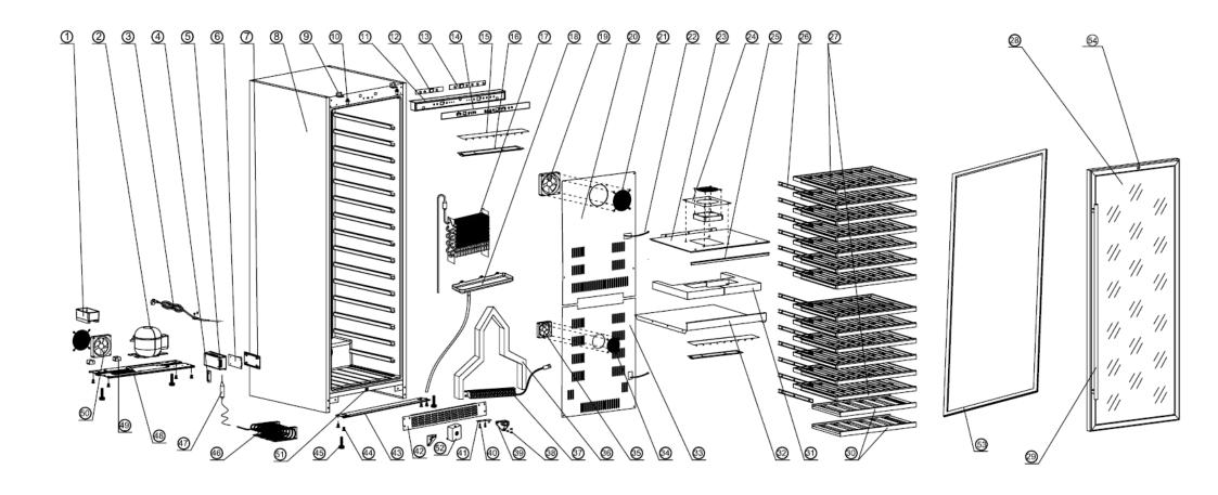
Exploded diagram and spare parts list (CE218) Rev.3
